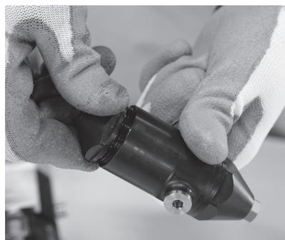
**Tightening torque: 15 N.m**
