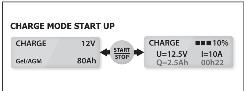
NB: When the charge ends (100%), if the battery remains connected the charger maintains the charge level of the battery by applying a floating voltage.
