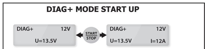
**Precaution :** If the screen displays a current greater than 10A, it indicates the battery is discharged. The device will start charging automatically. Check all electrical consumers are switched off on the vehicle. Wait until the current falls below 10A and then re-launch the diagnostic.
