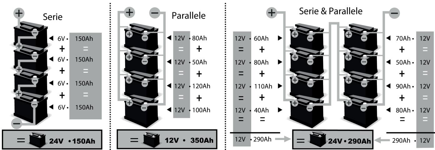
SCHÉMAS ÉLECTRIQUES / CIRCUIT DIAGRAM / SCHALTPLAN / DIAGRAMA ELECTRICO /
