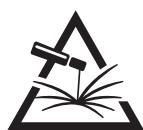
Protect the entire welding area. Compressed gas containers and other inflammable material must be moved to a minimum safe distance of 11 meters.
