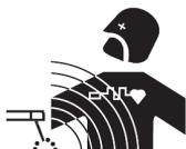
The electric currents flowing through a conductor cause electrical and magnetic fields (EMF). The welding current generates an EMF field around the welding circuit and the welding equipment.
