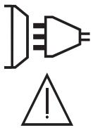
This equipment does not comply with IEC 61000-3-12 and is intended to be connected to private low-voltage systems interfacing with the public supply only at the medium- or high-voltage level. On a public low-voltage power grid, it is the responsibility of the installer or user of the device to ensure, by checking with the operator of the distribution network, which device can be connected.
