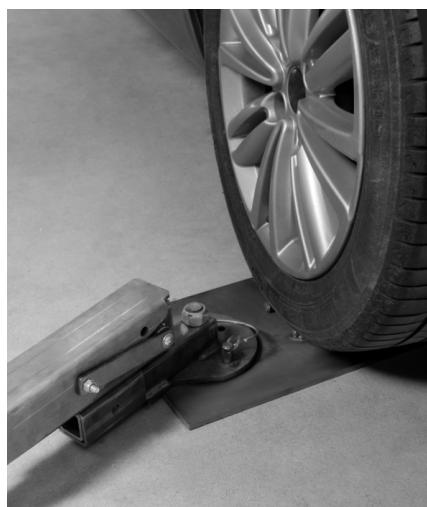
The DRAW ALIGNER PRO has a rotating pole to change the pull angle to suit the pulling situation.
