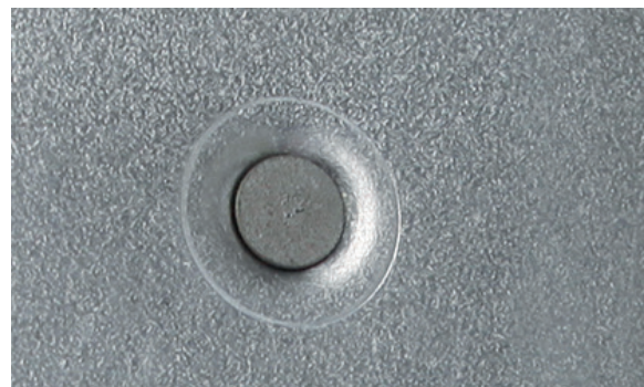
RESULT OF THE INSTALLATION OF SELF-PIERCING RIVET
