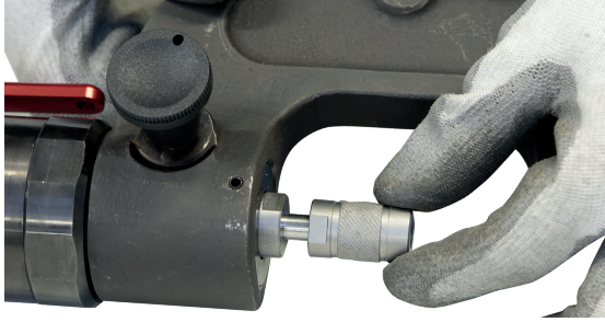
Using the screw, fasten the extension supplied with the arm.
