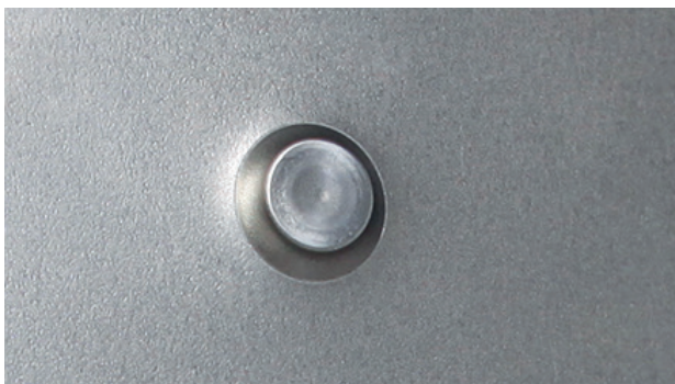
RESULT OF THE INSTALLATION OF SELF-PIERCING RIVET
