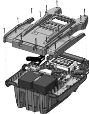
Disassemble the product is useful especially to replace batteries. Proceed as such :
